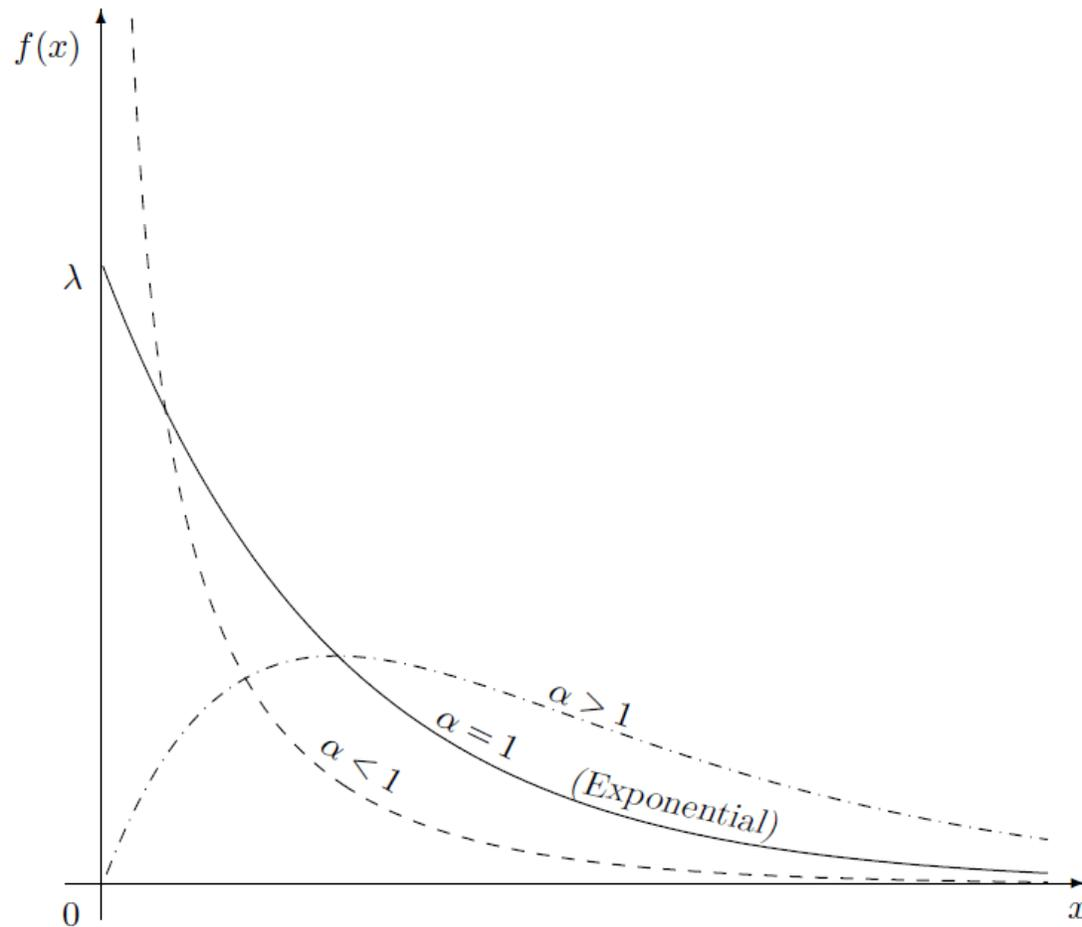
FIGURE 4.5: Gamma densities with different shape parameters  $\alpha$ .
